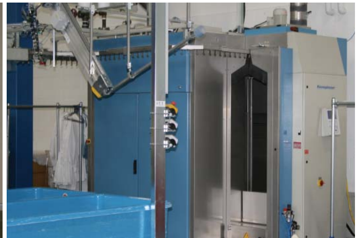
A view of a tunnel finisher used for healthcare garments in the plant
