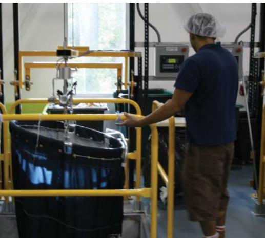
An employee inspects machinery that automatically moves slings of soiled goods to the wash aisle.
