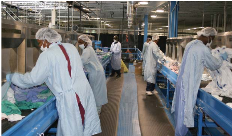
Employees sort soiled healthcare textiles into 48 hoppers. The goods then drop into slings that move to the wash aisle via an overhead rail system that automatically dispatches them when they reach a preset weight.
